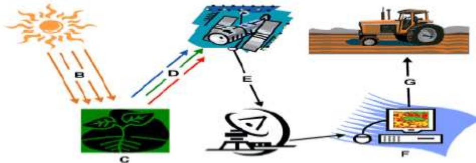
Figure 1: B is the EMR received from the Sun which is either absorbed or reflected by vegetation; D is the reflected radiation detected by sensor aboard satellite; E is the data transferred to ground station; F is the data being analyzed and information generated; G is the process of using the information on field for decision support. Such type of surveys and creation of maps is typically known as satellite mapping. Some of the advantages of satellite mapping are:
